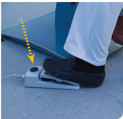
A foot switch is important for changing your light source. If your instrumentation provides optional changing between fixed vs. moving stroboscopic imaging modes, check which mode is being used and how to switch between the modes (see arrow).
