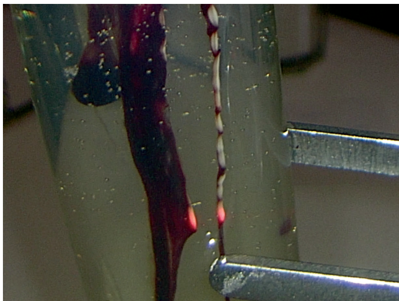
Figure 6: Blood strands within egg white in a glass test tube. KTP laser travels through glass test tube and egg white. All energy absorbed at blood, which coagulates immediately.
